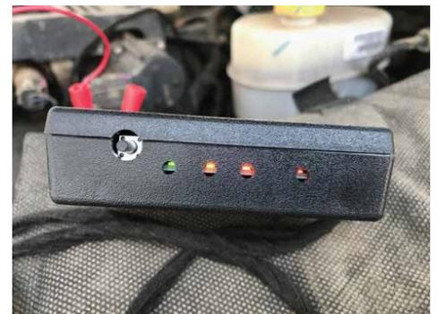
**FLASH CODES:** FLASH CODES ARE FLASHING LIGHTS ON EACH OF THE LED'S, THE NUMBER OF EACH ONE (RUNNING FROM LEFT TO RIGHT) WILL INDICATE THE ERROR EXPERIENCED.
