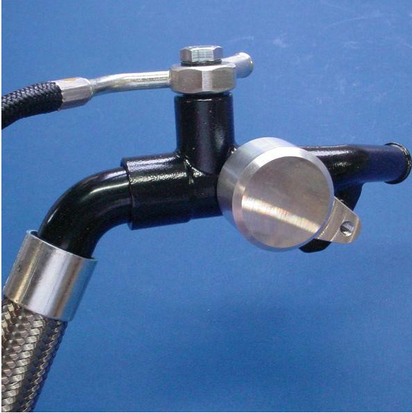
'13-'15 C&C Standpipe Cap Installed
